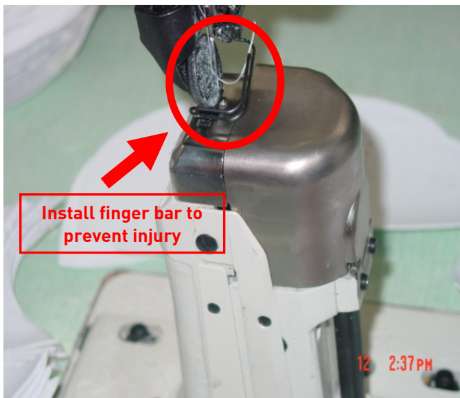
Figure 11.6 – Installation of Needle Guards on Sewing Machines
