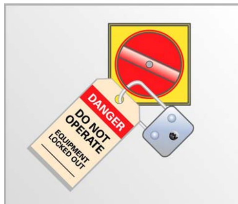
Figure 15.1 – Lockout/Tagout in Operation
