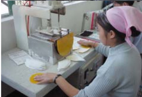
Machine with two-hand switch (does not work in one-hand modus)
