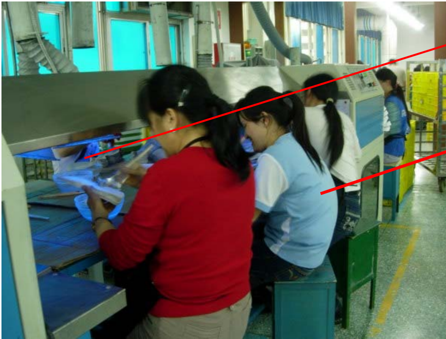
Figure 11.11 – No Protection against Chemical Exposure
