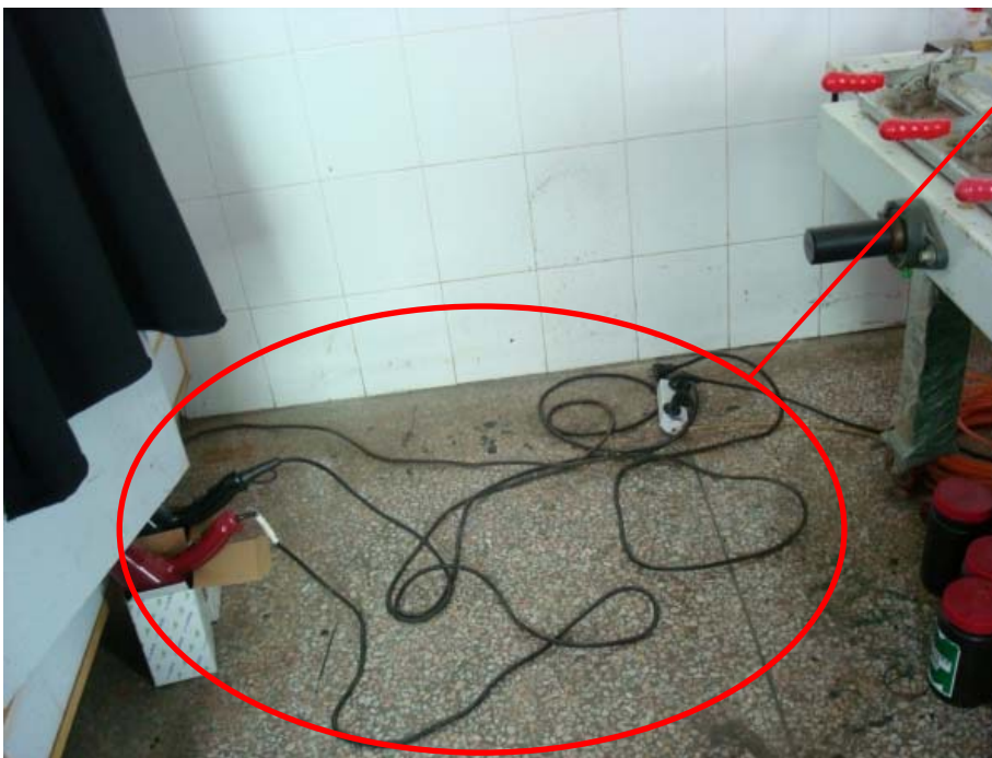
Figure 11.12 – Improper Storage of Hand Tools and Cabling
