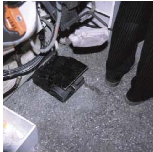
Protection over foot pedal of power driven machines
