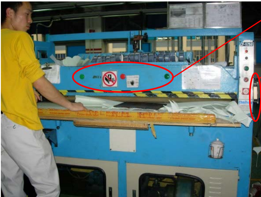
Figure 11.9 – Hand Switches and Infrared Devices Installed to Improve Machine Operation Safety
