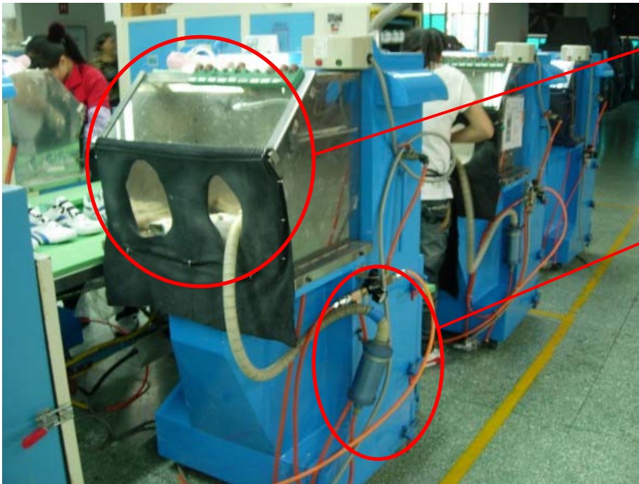
Figure 11.10 – Installation of Dust and Noise Minimisation on Machinery
