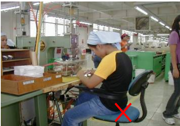
Figure 21.1 – Poor Work Position
