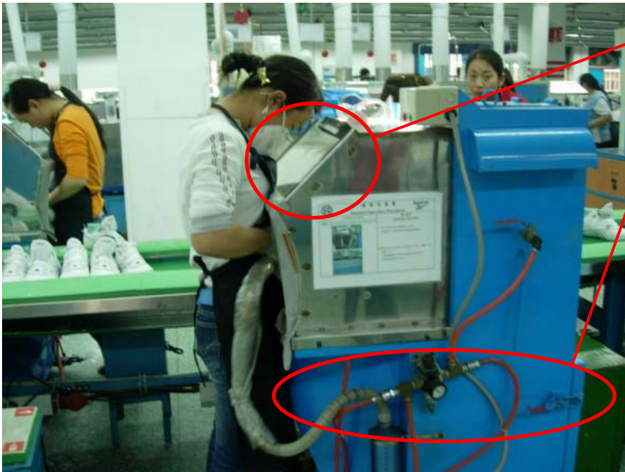
Figure 11.8 – Installation of Dust and Noise Protection on Machinery
