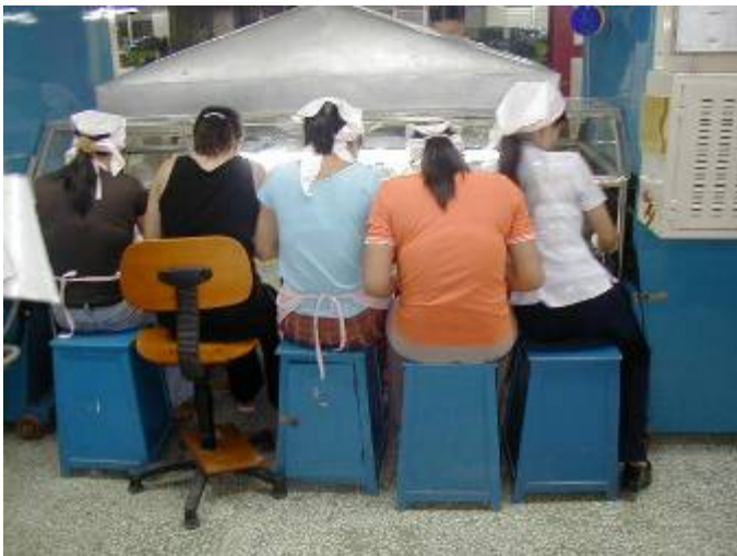
Figure 21.6 – Cramped seating results in concentrated compression and impact stress
