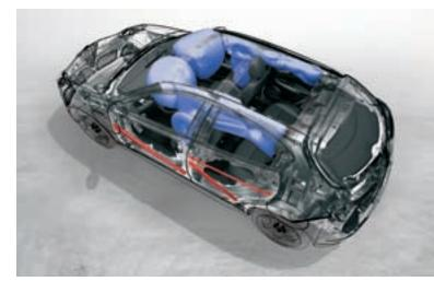
obtained on the position and speed of the obstacle enables the Pre-Crash function to pre-activate restraint systems (such as the electric seat belt pre-tensioners) to hold the vehicle's occupants in the best and most protected position for impact, and pre-alert protection systems (such as the airbags) to optimize timing and deployment.
