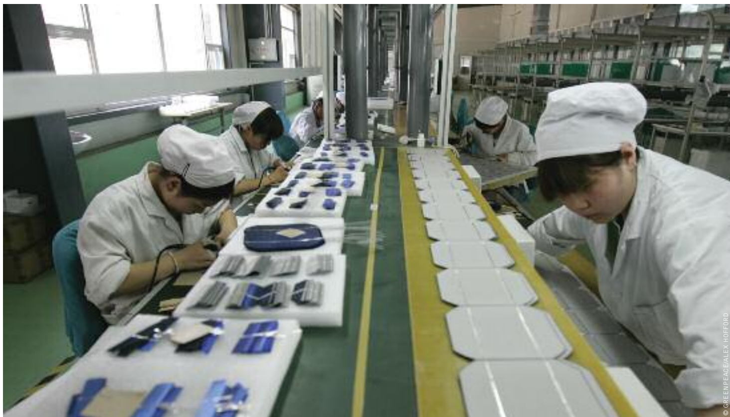
image SOLAR POWERED PHOTO-VOLTAIC (PV) CELLS ARE ASSEMBLED BY WORKERS AT A FACTORY OWNED BY THE HIMIN GROUP, THE WORLD'S LARGEST MANUFACTURER OF SOLAR THERMAL WATER HEATERS. THE CITY OF DEZHOU IS LEADING THE WAY IN ADOPTING SOLAR ENERGY AND HAS BECOME KNOWN AS THE SOLAR VALLEY OF CHINA.
