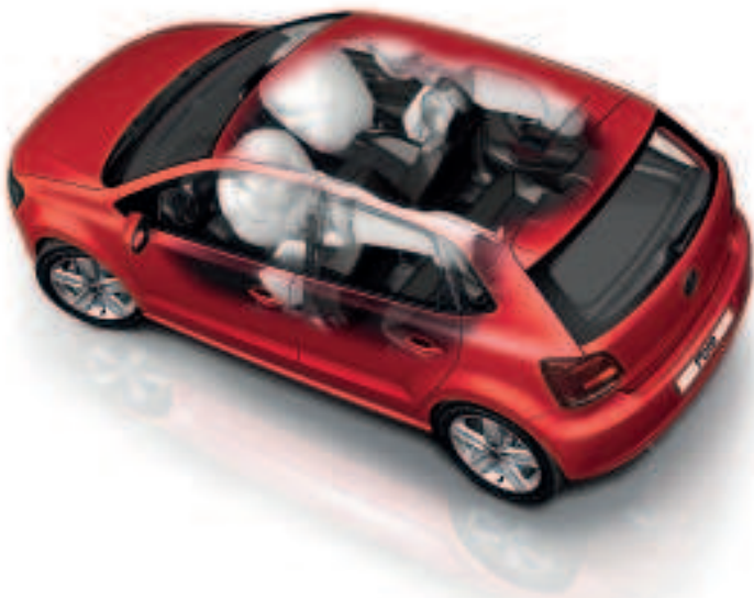
The airbag system in the new Polo.
